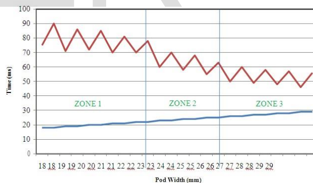
Figure 1 Graph of Pod Width in mm vs De-cortication time in milli second
